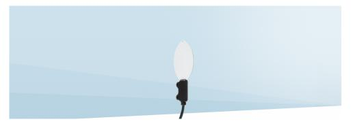
**Disease Prevention:** A Leaf Wetness Sensor is a crucial tool for disease prevention. Monitoring leaf moisture conditions allows farmers to keep track of moisture levels conducive to the development of fungal diseases such as mildew or rust. Early warnings enable appropriate countermeasures to be taken to prevent disease spread.
